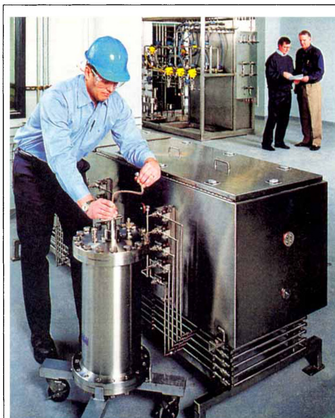
Figure 2. Largest cGMP validated Simulated Moving Bed unit operating in North America for chiral separations in the pharmaceutical industry. Located at Universal Pharma Technologies, LLC, North Andover, MA.
